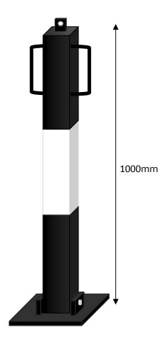
The SB.25 HP has a padlock facility at the top of the post (Padlock not supplied) complete with handles for easy operation.
