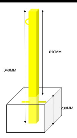
Our sunken economy post is a permanent fixture in the ground. Fitted with an eyelet, chain can be used to join multiple posts.
