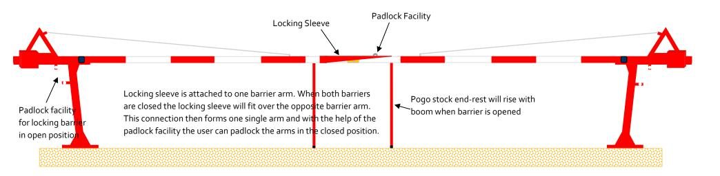
The SB.4 provides a low maintenance, cost-effective way of manually controlling access to unauthorised areas on a permanent or temporary basis. Durable and hard-working, this manual raise arm barrier has been manufactured for the last 32 years and compromises a robust and high quality pivot post, lockable end rest and aluminium boom.
